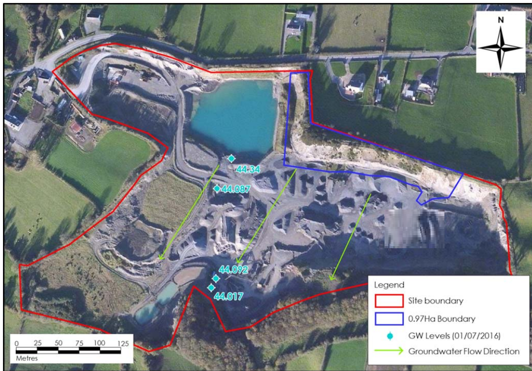
Figure 8-11: Local Groundwater Flow Direction Map
